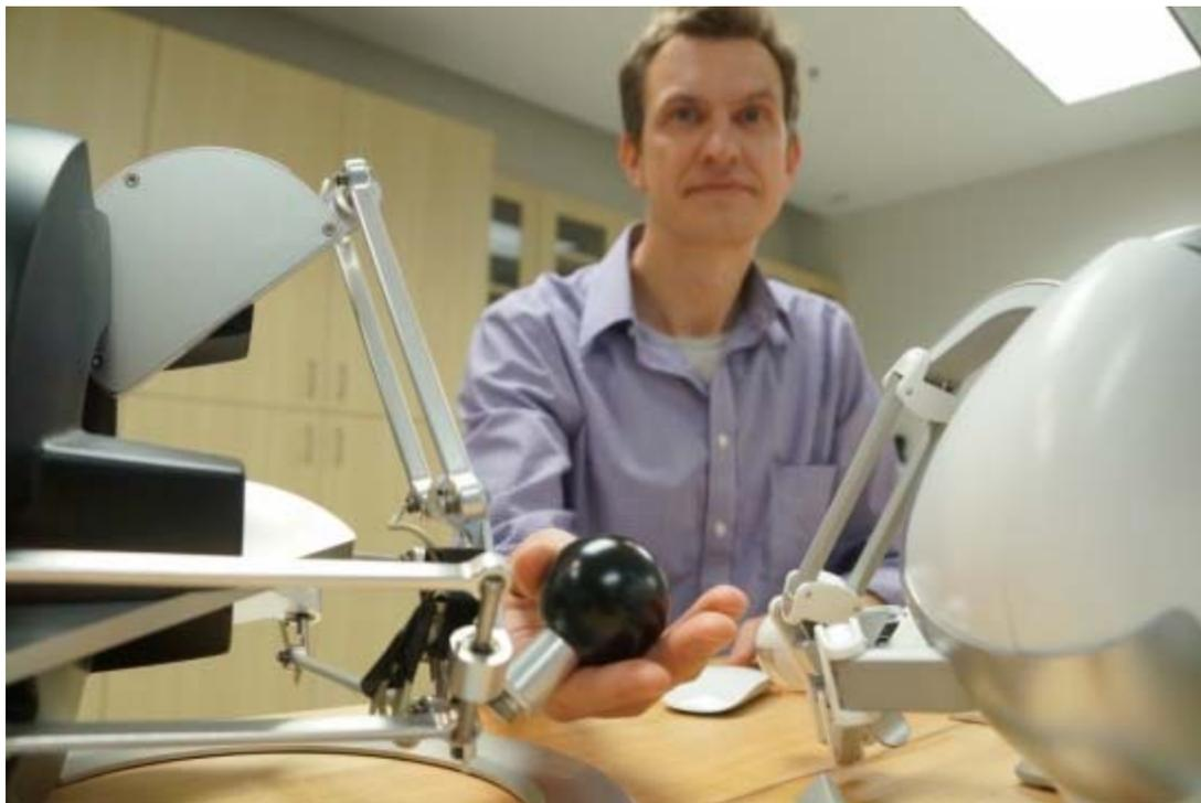
UCSB researcher Yon Visell and a device of the type used to simulate the forces felt by the hand when touching an object
