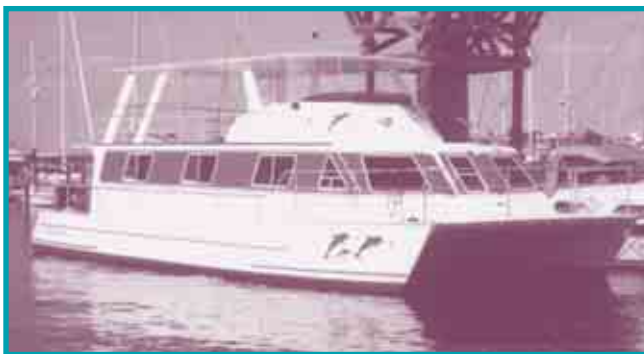
The Dolphin Star features six cabins, four-zone air conditioning, two complete heads with showers, a hot/cold on-deck fresh-water shower, a 500 gal./day desalination water maker, and a full galley.
